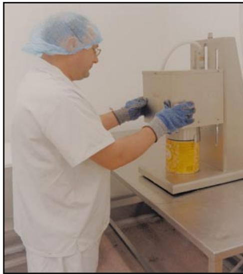
**Figure 24** Two-hand control, powered tin opener (avoiding repetitive hand movements)
