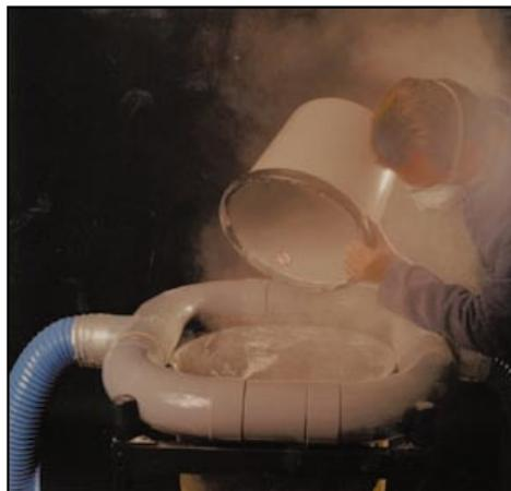
**Figure 17** Mixer with top-rim dust extraction turned off
