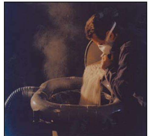
**Figure 18** Mixer with top-rim dust extraction turned on
