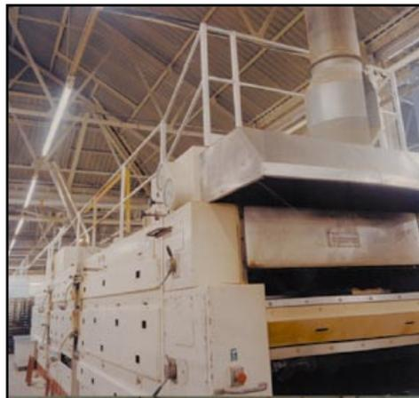
**Figure 67** Gas-fired equipment should be fitted with flame-failure devices
