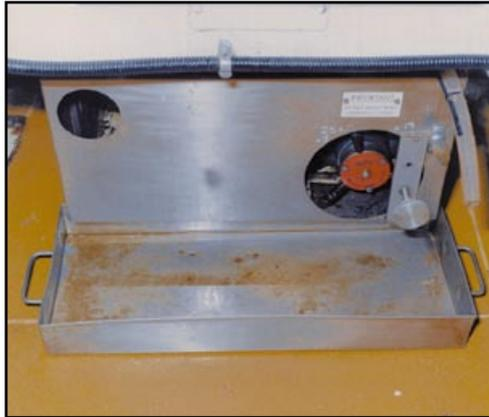
**Figure 27** Drip tray to catch divider oil and prevent floor contamination
