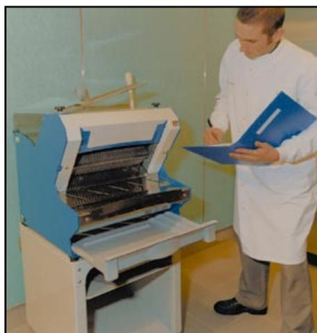
**Figure 8** Risk assessment on manually operated bread slicer
