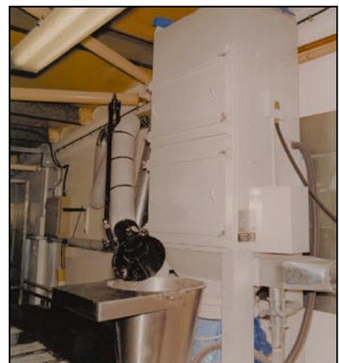
**Figure 13** Dust extraction at sack-tip point
