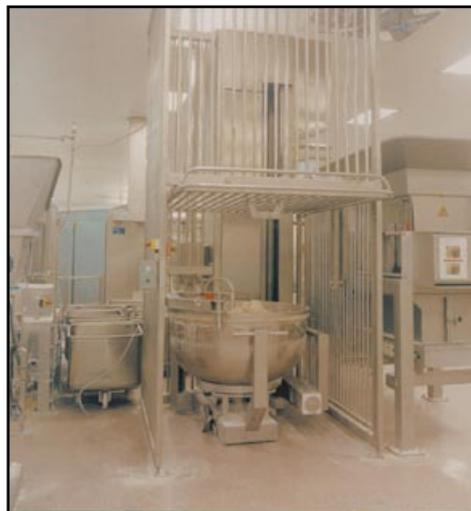
**Figure 48** Bowl hoist with fixed fencing around machine and interlocked, lift-up access gate
