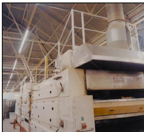
**Figure 42** Oven with handrails permitting safe oven-top access
