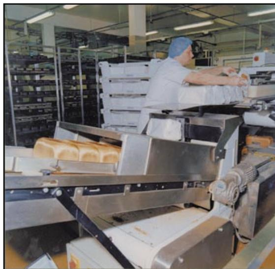
**Figure 50** Bread slicer with interlocked, infeed tunnel guard
