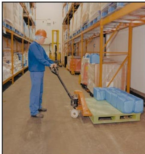
**Figure 26** Pedestrian-operated pallet truck transporting 12.5 kg blocks of fat
