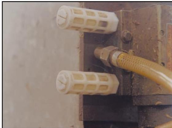
**Figure 57** Two silencers on pneumatic lines on a pie and tart shell machine. The noise level before the silencers were fitted was 113 dB(A). After they were fitted the noise level was reduced to 86 dB(A)
