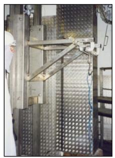
as before. Instead of hauling the carcass onto the second hook manually, the operator used the hoist to lower a section of the overhead rail. The loose end of the rope was fitted over the hook. Using the hoist, the rail, hook and carcass were raised up to a comfortable height for cutting through the rest of the carcass until the two portions were separated.
