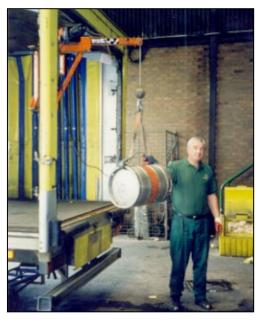
power source and a fitment bracket. The hoists allow the kegs to be lifted direct from the floor onto the vehicle by means of attached straps and hooks. The company has purchased several hoists, each costing approximately £1500 and the plan is already under way to equip vehicles at each distribution depot.
