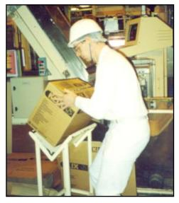
back postures seen when tall people were working at the fixed-height packing stations were also identified as risky. Twisting to place the filled box onto the conveyor belt also presented a risk of back injury.
