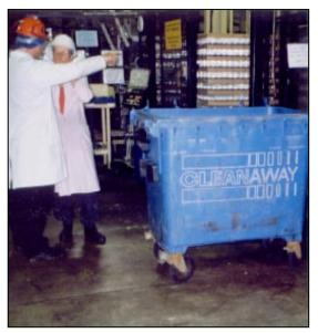
The company bought six mini-skips to replace the wheelie bins were placed at various points on the line, at an approximate cost of £650 each. When the mini-skips are full they are lifted by a fork-lift truck and transported to an outside waste dock, where they are emptied.
