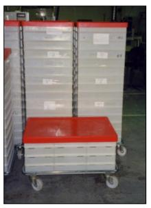
had no sharp edges, was easy to use for this company's product, and cost £32. It also had a metal ring which helped prevent the stacks from sliding off the trolley if it hit an obstruction on the floor. The company purchased 320 of these trolleys, to replace the wooden ones. The total cost was approximately £10 000.
