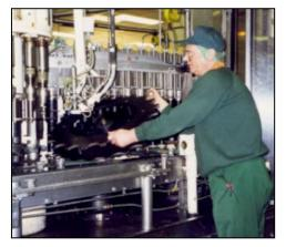
The company replaced the existing star wheels with lightweight versions. The new star wheels have all unnecessary material taken out of them (eg the centre of each wheel is now cut out). They contain only half the material, weighing only 10 kg, but retain rigidity. Replacing the star wheels cost approximately £4000.
