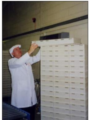
The weight of each tray was between 5 and 10 kg, and the dimensions of each tray were 75 x 40 x 10 cm. The total weight of a stack of trays could be as much as 200 kg. Trays were often overloaded, and/or asymmetrically loaded so they were heavier at one end than the other. There were no (designed) handholds on the trays, although the sides were relatively easy to grip. The total height of a stack of 20 trays and a trolley was 215 cm.
