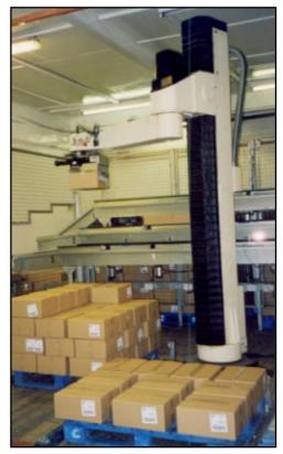
The company installed a 'pick-and- place' robot which lifts the boxes off the conveyor and palletises them to the correct height, pattern and variety.
