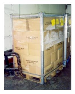
processing, the pallets were transported to a process line. An operator removed the boxes from the pallet, carried them 5-7 m and then emptied them manually onto the line. The box would then be broken down and placed in a skip. Twenty operators were required to carry out these tasks.
